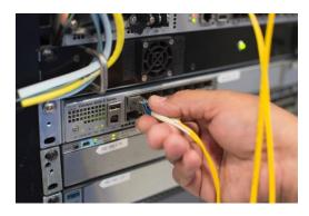
The last step in the part qualification process is coding and application testing in a wide variety of platforms. Depending on the form-factor, a part will be tested in as many as 50 different platforms or combinations of chassis, controllers, line cards and operating system revisions from multiple OEM's. Test results are recorded for each configuration and added to DHD's part compatibility matrix.
